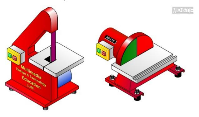
An illustration of a linisher and a disc sander is shown above. Describe the safety checks that you would carry out before starting to use either of the two machines.
