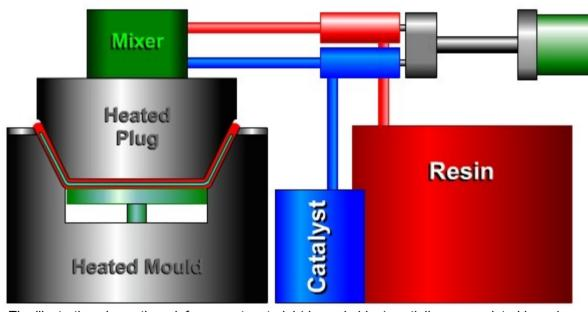
The illustration shows the reinforcement material (drawn in blue) partially encapsulated in resin
