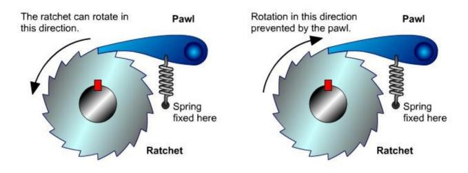
A pawl is a metal part that rests on the ratchet. As the ratchet rotates, the pawl drops onto each of the steps on the ratchet rim, preventing the ratchet from turning in the direction of the pawl.
