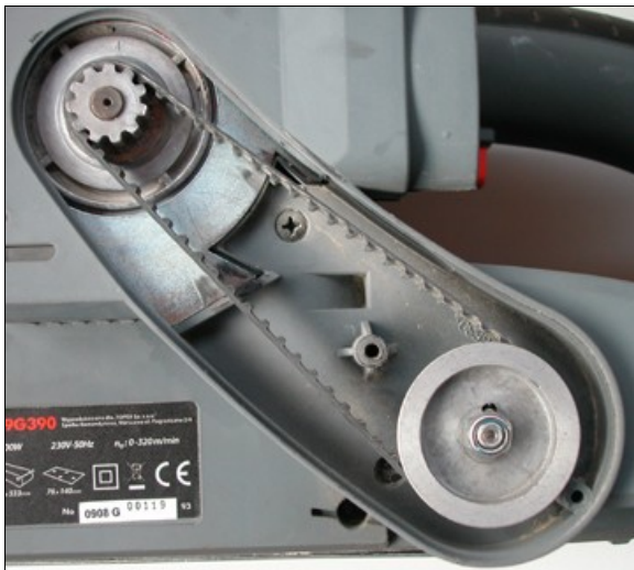
Toothed belt and pulleys used on a belt sander
