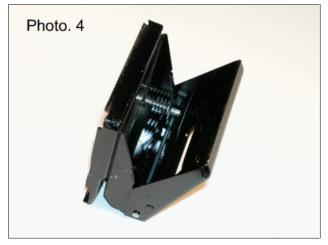
This view of the paper punch shows that the black sheet metal parts are made from three separate pieces of metal.
