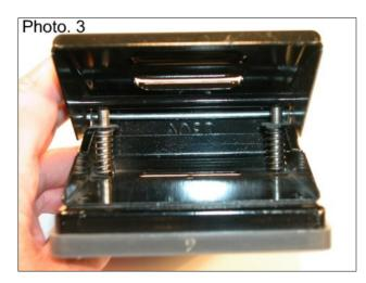
This view of the paper punch shows the punches, the springs and other components.
