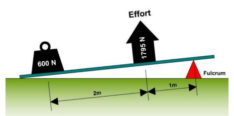
There is a 600N load acting on the lever 3 metres from the fulcrum so the anticlockwise moment is 1800Nm. There is a 1795N effort acting on the lever 1 metre from the fulcrum so the clockwise moment is 1795Nm. In order to lift the load, an effort greater than 1800Nm must be applied or the distance from the effort force to the fulcrum must be increased.
