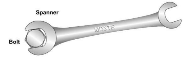
The moment = the size of the force (N) multiplied by the length of the lever (m).
