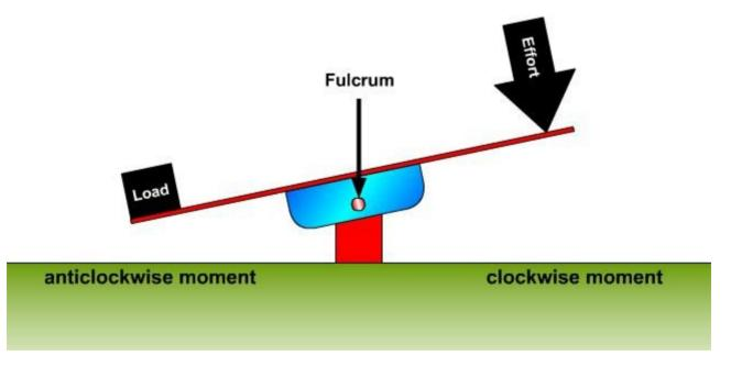
A load on one end of a see-saw will create a turning effect about the fulcrum called a moment. A load is an example of a force.
