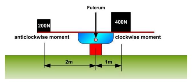
The diagram above illustrates two unequal loads placed on the seesaw.
