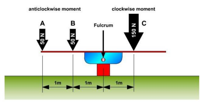
In the example above, two 50N loads are placed on one side of the seesaw and a 150N load is placed on the other. The see-saw is balanced because the clockwise moment is equal to the sum of the anticlockwise moments, i.e.
