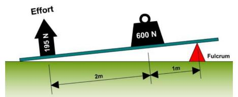
There is a 600N load acting on the lever 1 metre from the fulcrum so the anticlockwise moment is 600Nm. There is a 195N effort acting on the lever 3 metres from the fulcrum so the clockwise moment is 585Nm. In order to lift the load, an effort greater than 600Nm must be applied or the distance from the effort force to the fulcrum must be increased.
