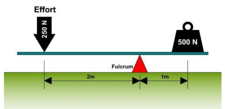
There is a 500Nm anticlockwise moment and a 500Nm clockwise moment, so the lever is in equilibrium. In order to lift the 500N load higher, the effort must be increased or the distance from the effort force to the fulcrum must be increased.
