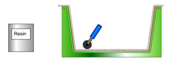
Once again an exothermic reaction occurs causing the resin to cure and harden and bond with the gel coat layer.
