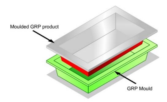
The mould is first checked for defects, any scratches etc. are filled. The mould is then polished with a wax polish to a very smooth, high quality finish. Next, a very thin film of a liquid release agent is applied to the inside of the mould. The wax and the release agent are there to prevent the glass fibre product from sticking to the mould.
