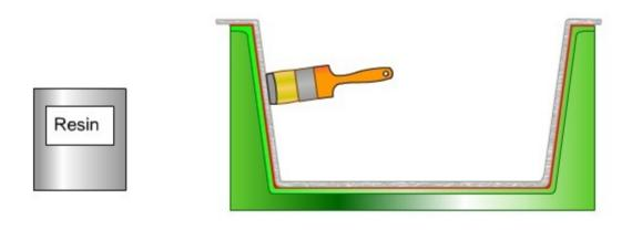
A roller is used to ensure that the resin is spread evenly all over the mould. After rolling, the glass reinforced composite is left to cure and harden.
