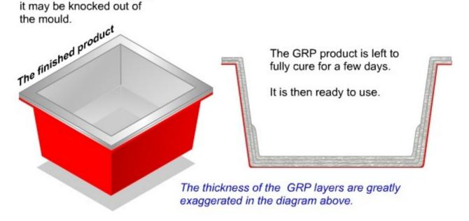
When the product has fully cured, it may be removed from the mould. The coloured gel coat that was on the inside of the mould is now the exterior covering of the GRP product.
