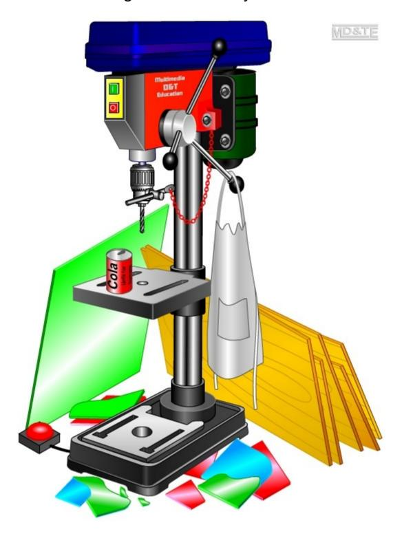
Safety exercise: identify the hazards on and around the drilling machine
