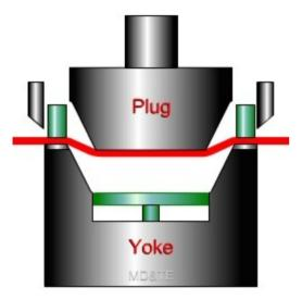
The plug pushes the SMC into the mould. Heat from the mould cures the SMC.
