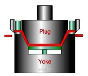
When the SMC has cured, it is ready to be trimmed and ejected from the mould.
