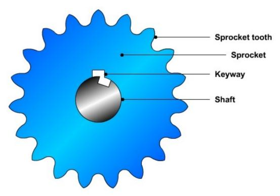
Chain and sprocket mechanisms perform the same task as a belt and pulley system, i.e. they transfer motion and force from one shaft to another. A belt can slip on a pulley but the teeth on the sprocket prevent the chain from slipping. A chain and sprocket is used wherever a positive, non-slip drive is required, e.g. bicycles, motorcycles, forklift mechanisms, and the camshaft drives in car petrol engines.
