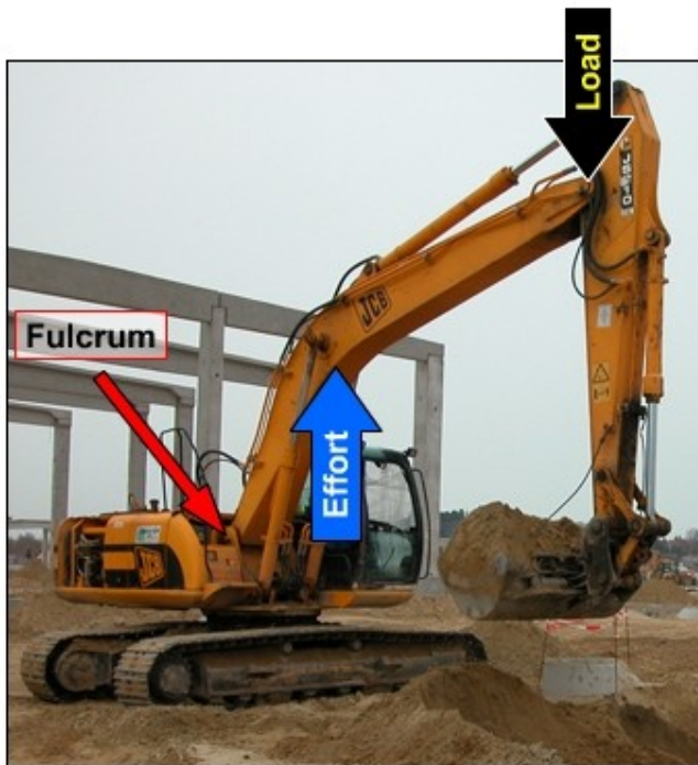
Class 3 lever: the lower digger arm
